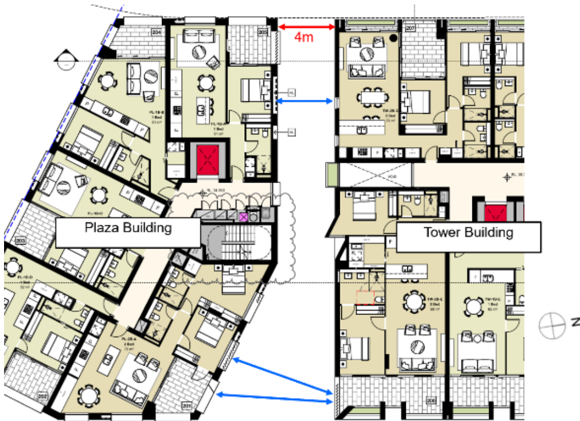
Figure 74: Bedrooms within the Plaza Building have highlight windows where they face narrow, vertically oriented windows for living areas of the Tower Building (blue arrows in Figure 75 below). Privacy screens are provided to prevent mutual overlooking between balconies and bedroom windows.
