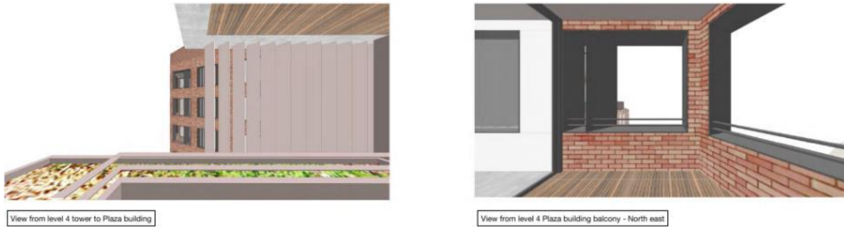
Figure 76: Angled louvres are proposed to mitigate impacts caused by mutual overlooking between balconies. Images include views from Tower Building balconies (left) and the Plaza Building (right).
