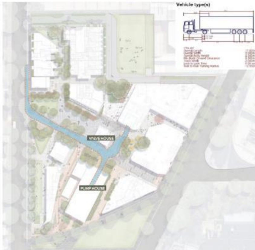
Figure 20: Swept paths for Sydney Water vehicles. Amended swept paths, showing Sydney Water articulated vehicles servicing the Pump House and Valve House from Young Street only. A new roller door will be installed on the northern wall of the Pump House, in the event McEvoy Street is resumed for road works.
