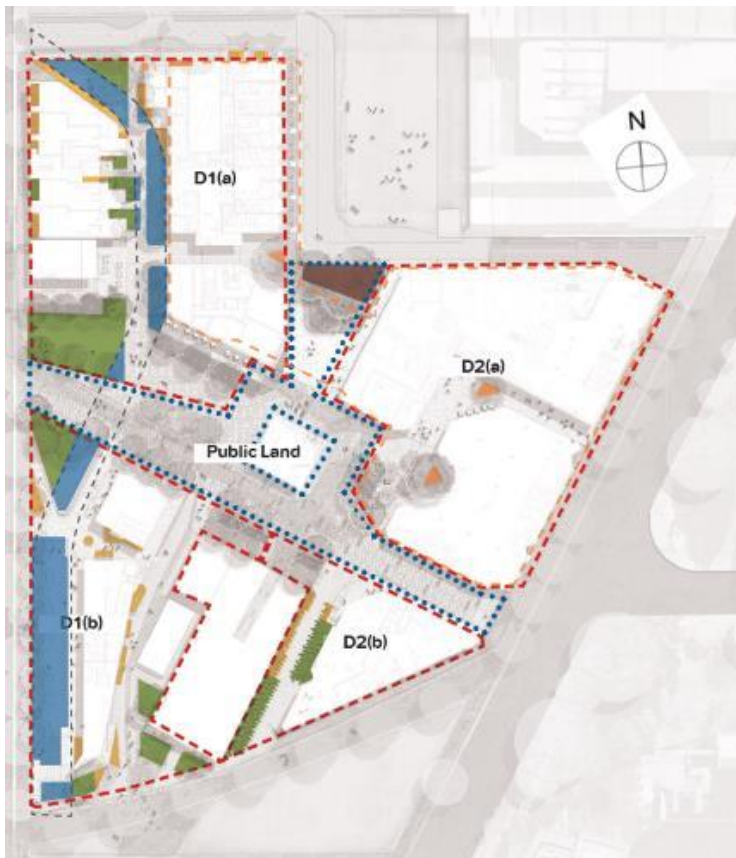
Figure 87: Site-wide deep soil zones, showing compliant 3m depth areas (shaded green), additional areas less than 3m (shaded orange), and above Sydney Water culverts (shaded blue), extracted from Landscape DA Package
