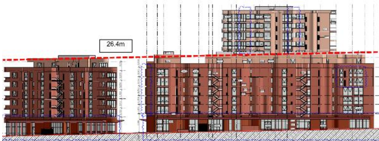
Figure 65: Elevation plan showing parts of the Bourke Street North and Bourke Street South Buildings that are proposed to exceed the height of buildings standard, including parapets and roof level plant enclosures
