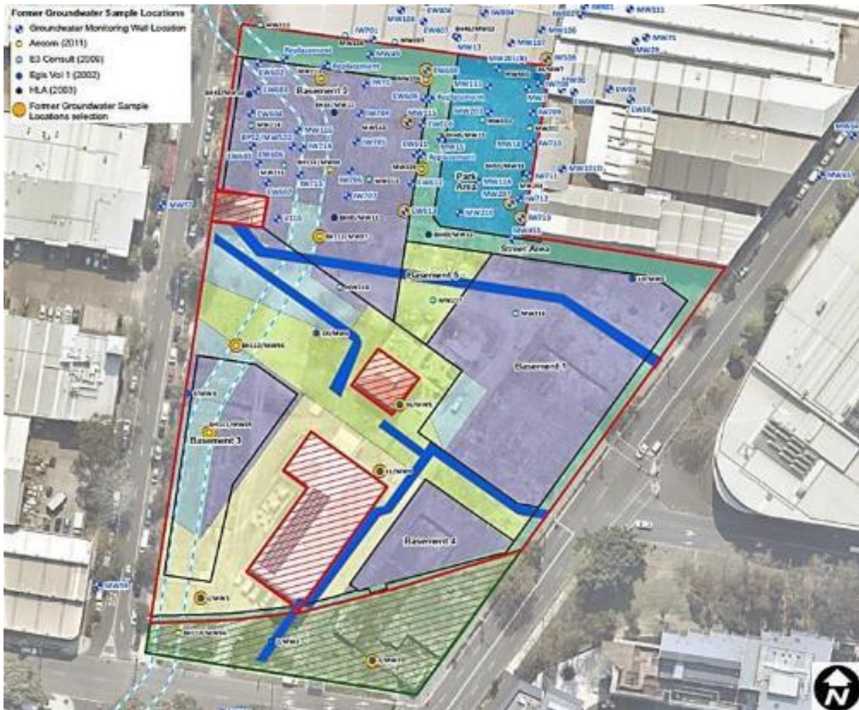
Figure 55: Blue and white markers indicate location of wells required to monitor groundwater
