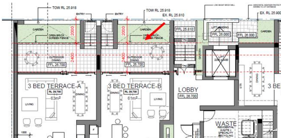
Figure 72: Amended ground floor plan showing loggia has been deleted, replaced by 2m landscape setbacks, clear to the sky for the full height of the building. Balconies have been made larger facing Young Street (red arrow).
