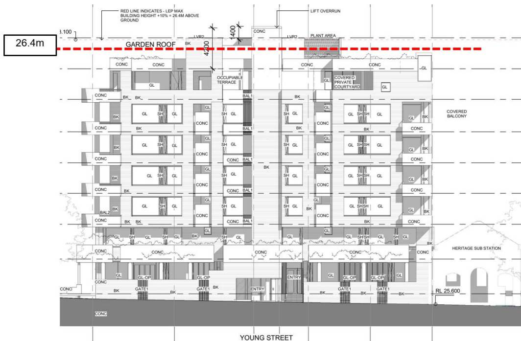
Figure 62: Elevation drawing showing Young Street North Building relative to the height of buildings standard (red dotted line)
