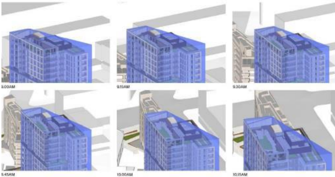
Figure 60: The part of the building that exceeds the height of building standard will cast shadow on the roof of the Tower Building
