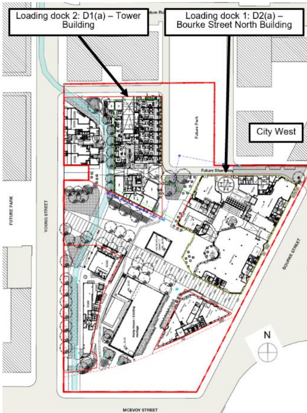
Figure 21: Second loading dock now provided beneath the Tower Building, relieving pressure from the original loading dock in the Bourke Street North Building, close to the City West development
