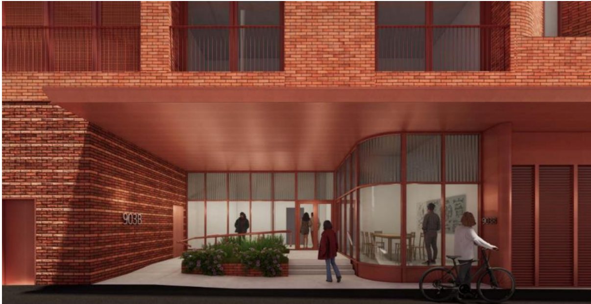
Figure 81: Extract from Bourke Street North Building drawing, showing the lobby off the shared zone in north-east corner of the Bourke Street North Building being set in, to permit additional surveillance over the shared zone
